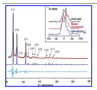
Figure 2. Experimental (black) and calculated (blue) PXRD patterns for COF-202 including Le Bail fitting (red) and the difference plot (turquoise). <sup>11</sup>B NMR traces of COF-202, model compound C, and starting material are shown in the inset.
