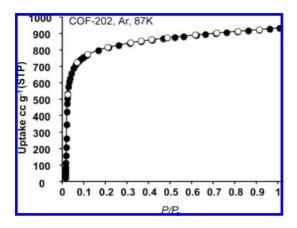
Figure 3. Gas adsorption isotherm for COF-202 with adsorption desorption points represented by closed circles and open circles, respectively.
